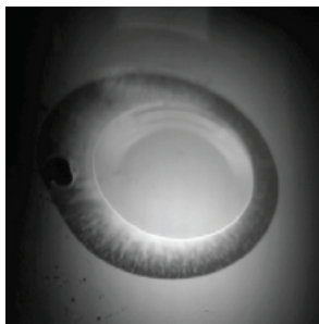
Sequence of grey scale images that show dimpling of the liquid-liquid interface, localised film rupture and spreading dendrites. Note the lifting of the droplet at one end to facilitate film drainage.
